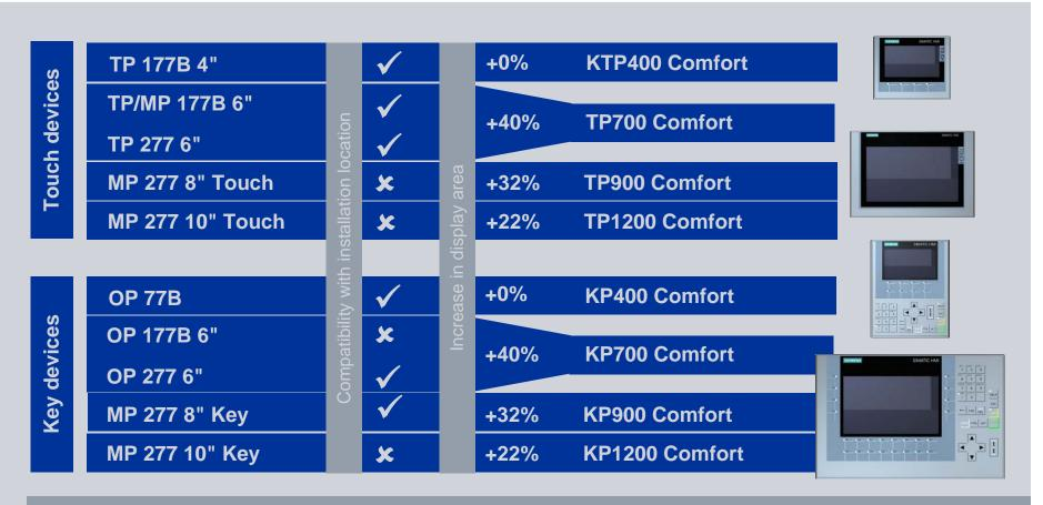
The widescreen displays increase usable display area by up to 40 percent when compatible with the installation location.
