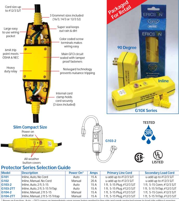
\* Power on function : Auto = GFCI comes on immediately upon power being applied to line side and sends protected power to load side without pressing buttons. Manual = RESET/START button must be pressed to send protected power to Load side of GFCI. All GFCIs must be RESET if a trip condition occurs. No automatically resetting functions are possible after a trip condition.
