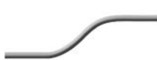
Offset bend Changes the conduit plane to clear obstacles or to rise up from a wall to enter a junction box
