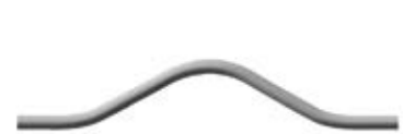
Three bend saddle Allows conduit to clear an obstacle, maintain alignment and appearance
